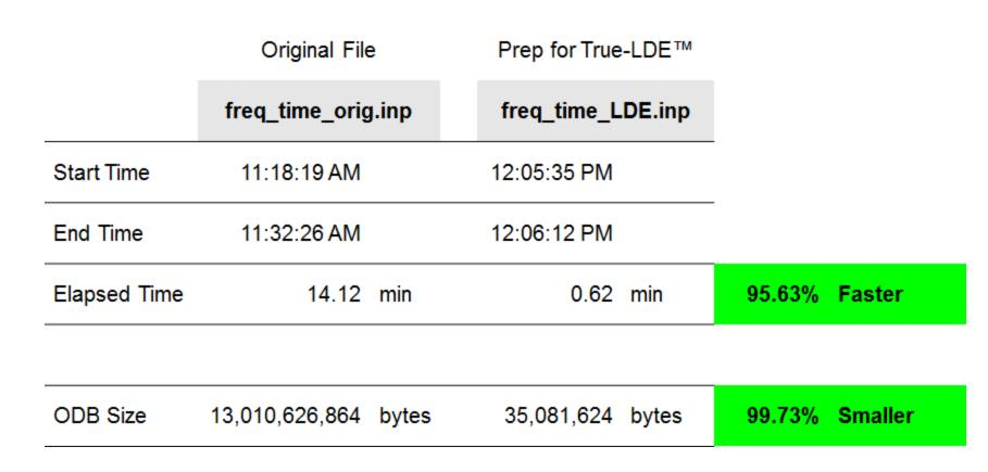
When solving a linear dynamic response for use with True-LDE, FEA solution time is significantly faster because of the greatly reduced output in the response solution.
